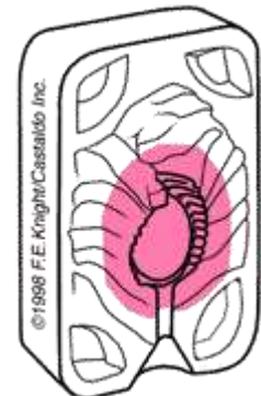
"Center-Only" Mold Made of No Shrink Pink Rubber and White Label or Gold Label
