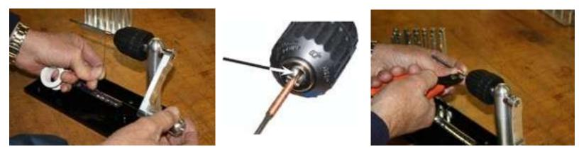
3) Remove the coiled wire from the mandrel. The end that is inserted into the arbor hole may be clipped or lifted out. Clip off or bend either end that may be sticking out above the coil. This will insure that the coil will lay flat in the V bed of the coil holder
