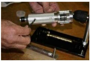
9) Place the cover over the coiled wire and replace the hold down nuts. Hold the cover down with your fingers right over the coiled wire. Tighten the nuts firmly but not excessively. Be certain that the cover is level over the coiled
