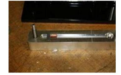
6) Place the coiled wire into the coil holding devise making certain that the lubricated side of the coil is up and the coil butts up against the stopping bracket.
